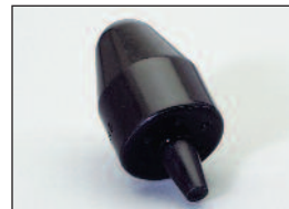
9.9166 Universal round pull thru bump stop. 2 9/16" tall x 1 3/4" dia. designed to fit 1/2" hole dia. x 3/32" thickness. 2 per set.
